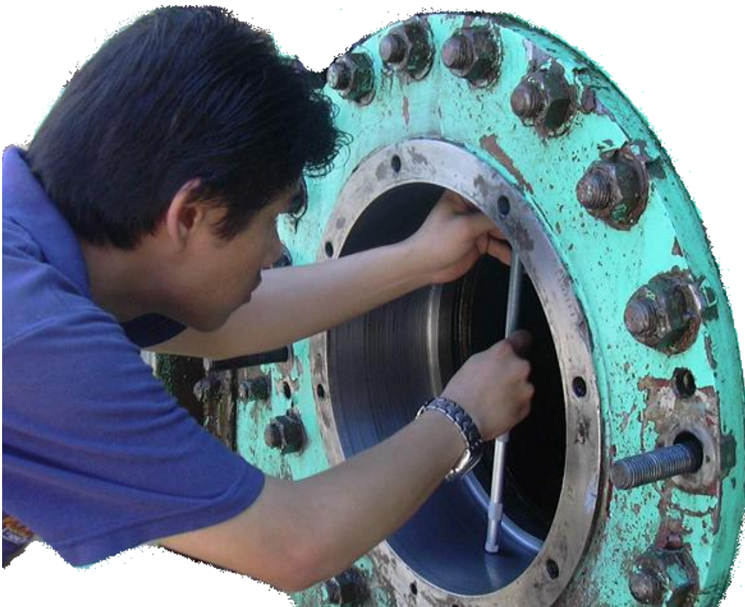
Measuring a bearing housing fitting tolerance with an internal micrometer
